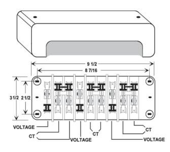
SWITCH DIMENSIONS 9 1/2" X 3 1/2" X 2 3/4" COVER DIMENSIONS 10 1/8" X 4 5/8" X 3 1/8"
