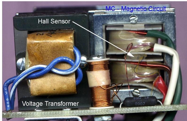
PC5 series watt transducer instantaneous input measuring circuit.
