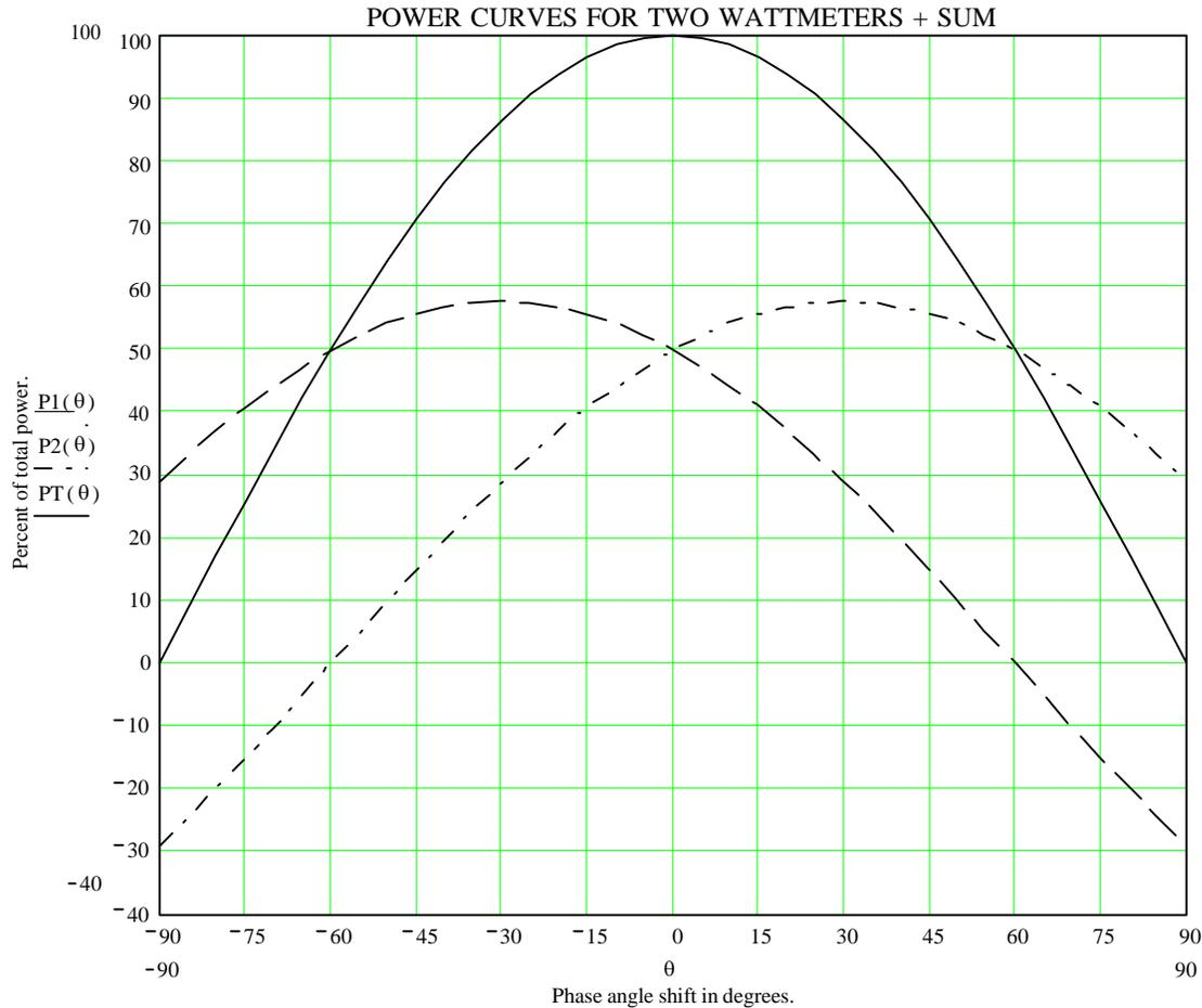
In the graph above the solid line represents total power. The dashed line represents the power as measured from phase A to phase C. The dash-dot line represents the power as measured from phase B to phase C. Some things to note:
